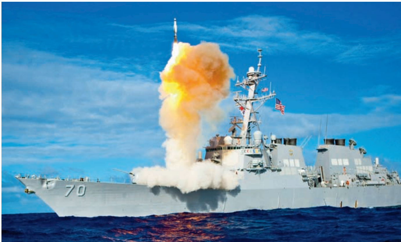
DEFENSIVE CAPABILITY: USS Hopper launches a RIM-161 Standard Missile (SM) 3 during a successful at-sea test firing to intercept a ballistic missile
